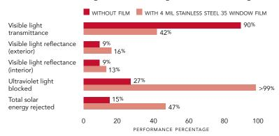
All performance results are based on the film installed on the inside surface of 1/8" (3mm), 1/4" (6mm), and 1/8"+1/8" (3mm+3mm) thick, clear glass.
