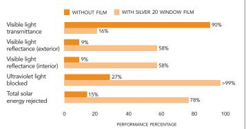
All performance results are based on the film installed on the inside surface of  $4\rm mm$  and  $4\rm mm+4\rm mm$  thick, clear glass.
