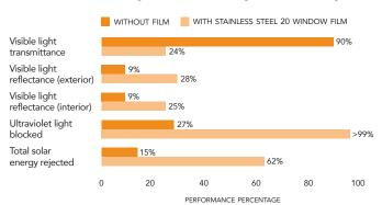
All performance results are based on the film installed on the inside surface of 4mm and 4mm+4mm thick, clear glass.
